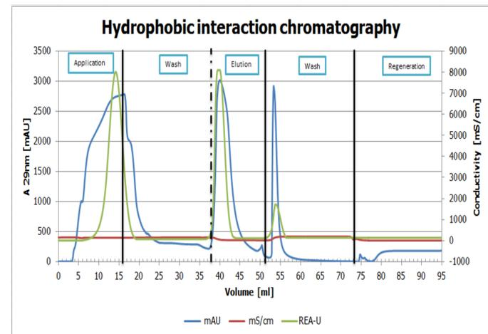
Fig. 2: Hydrophobic interaction chromatography using an ÄKTA Explorer system (GE-Healthcare).
